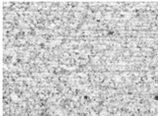
FINE ADZE min thickness - 1" / 25 mm
